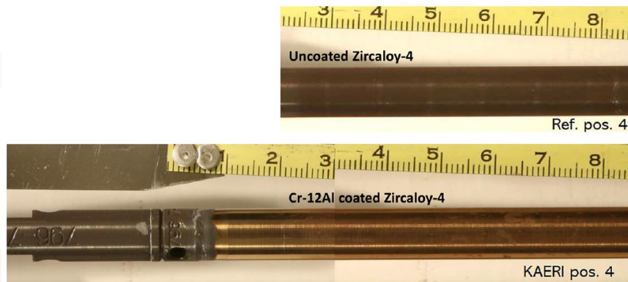
FIG. 10 Appearance of the Zircaloy-4 cladding and Cr-12Al-coated cladding tube after one-cycle irradiation test in the Halden reactor.
